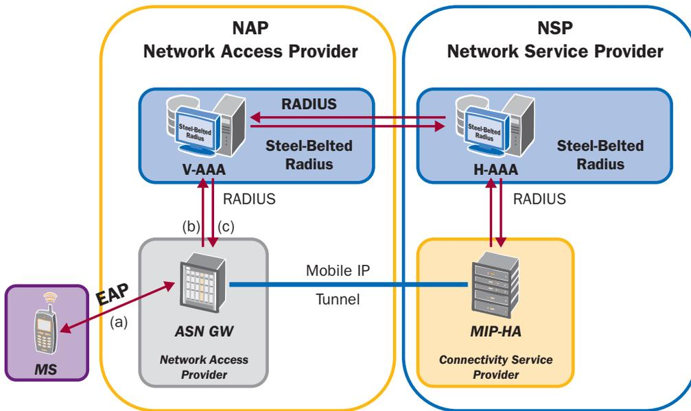
Figure 1: WiMAX Authentication Using Juniper Networks SBR Carrier AAA Server
